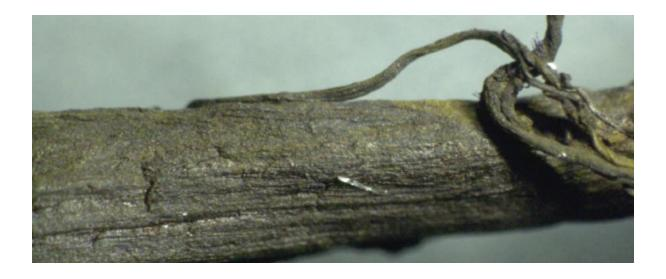
A laminated (layered) structure is clearly visible, as are crystalline deposits.
